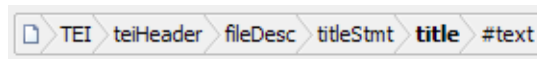
Figure 3-3. The node path bar showing that caret is currently inside a text node ( #text ), itself contained in a title element, itself contained in a titleStmt element, and so forth up to the root TEI element
